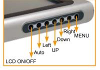
OSD Keypad is designed for AFL-15M/17M/19M
